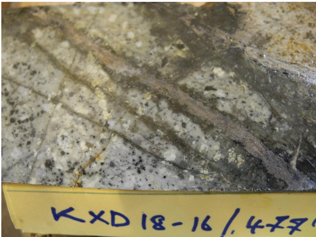
Plate 17: DDH KXD 18 – 16 at 477 feet (145m) downhole. A metasomatic endoskarn vein stockwork “vein” & “veinlet” system with the largest vein cored by pinkish brown andradite garnet. Note the irregular and embayed margins between the ore garnet and the yellowish green selvedge of scapolite which also has a ragged contact with the enclosing partially bleached and silicified GPB.
