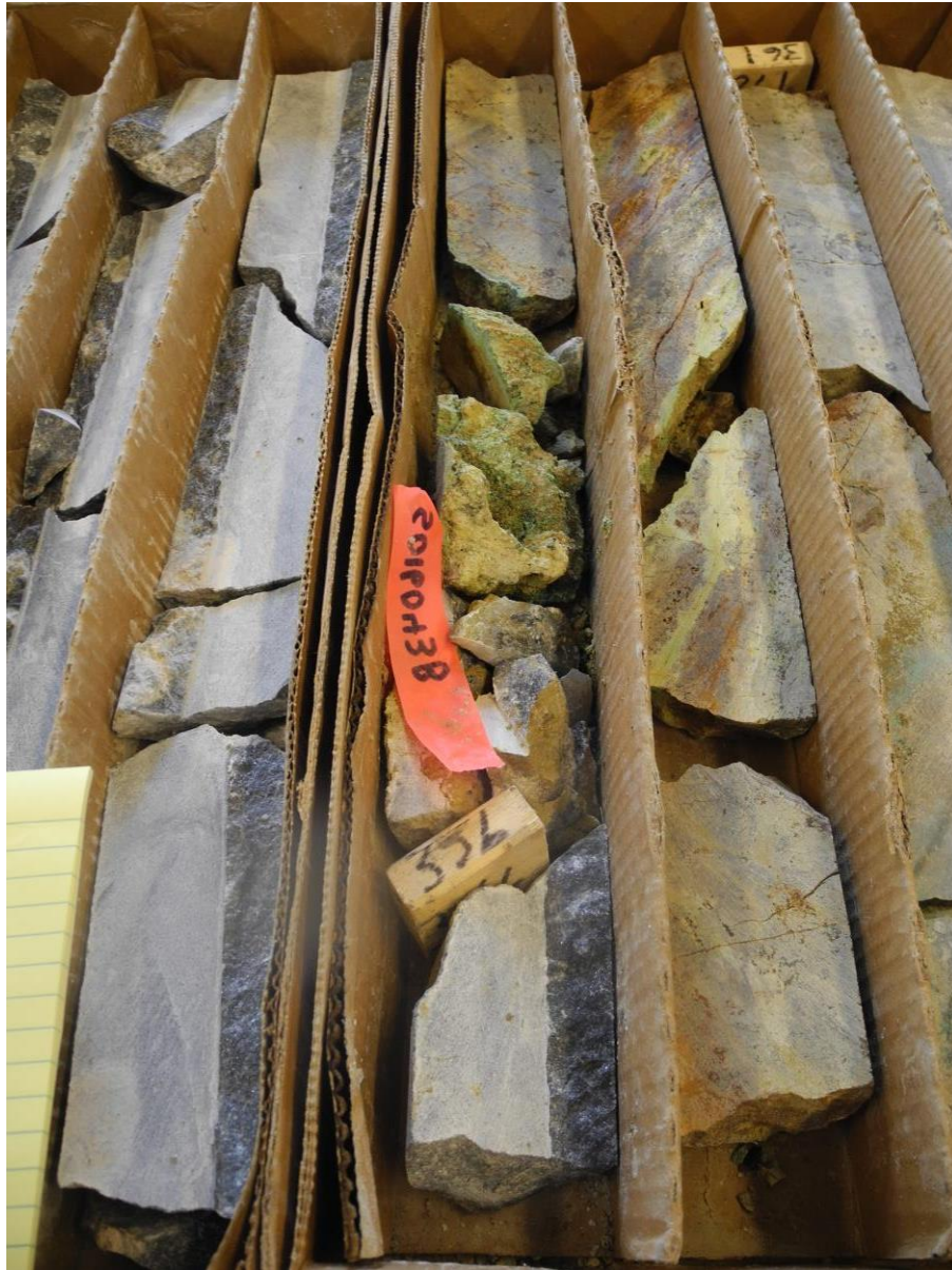
Plate 11: DDH S016B at 356 feet downhole (108.22m). This core tray shows the contact zone between the wollastonite marble skarn to the left and the somewhat oxidized and limonite stained (iron sulphide mineralized) calcic exoskarn (garnet plus pyroxene) to the right; photograph by author.
